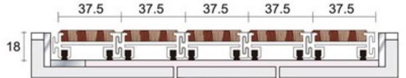
凹槽内铺设 Installation in groove
